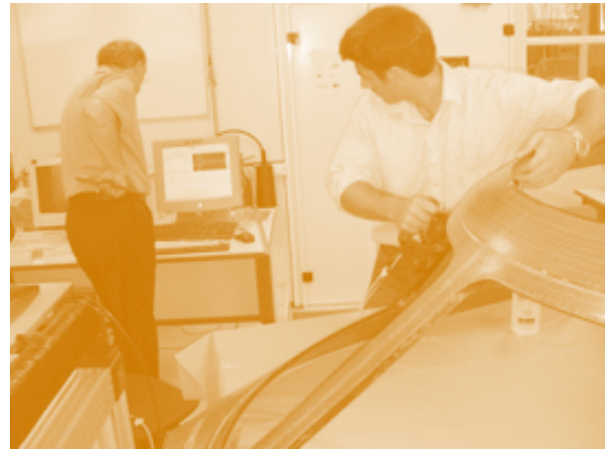
Image shows inspection of an advanced composite at Dassault Aviation, using an M2M system to drive the linear array probe. Used by permission.
