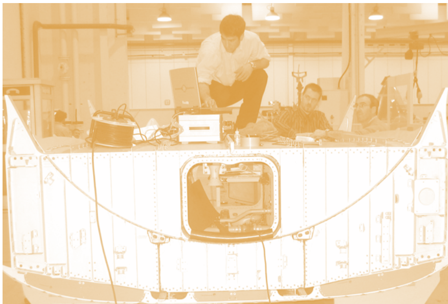
On-site inspection of T-section stiffeners, using M2M phased-array unit. Image courtesy of Dassault Aviation.
